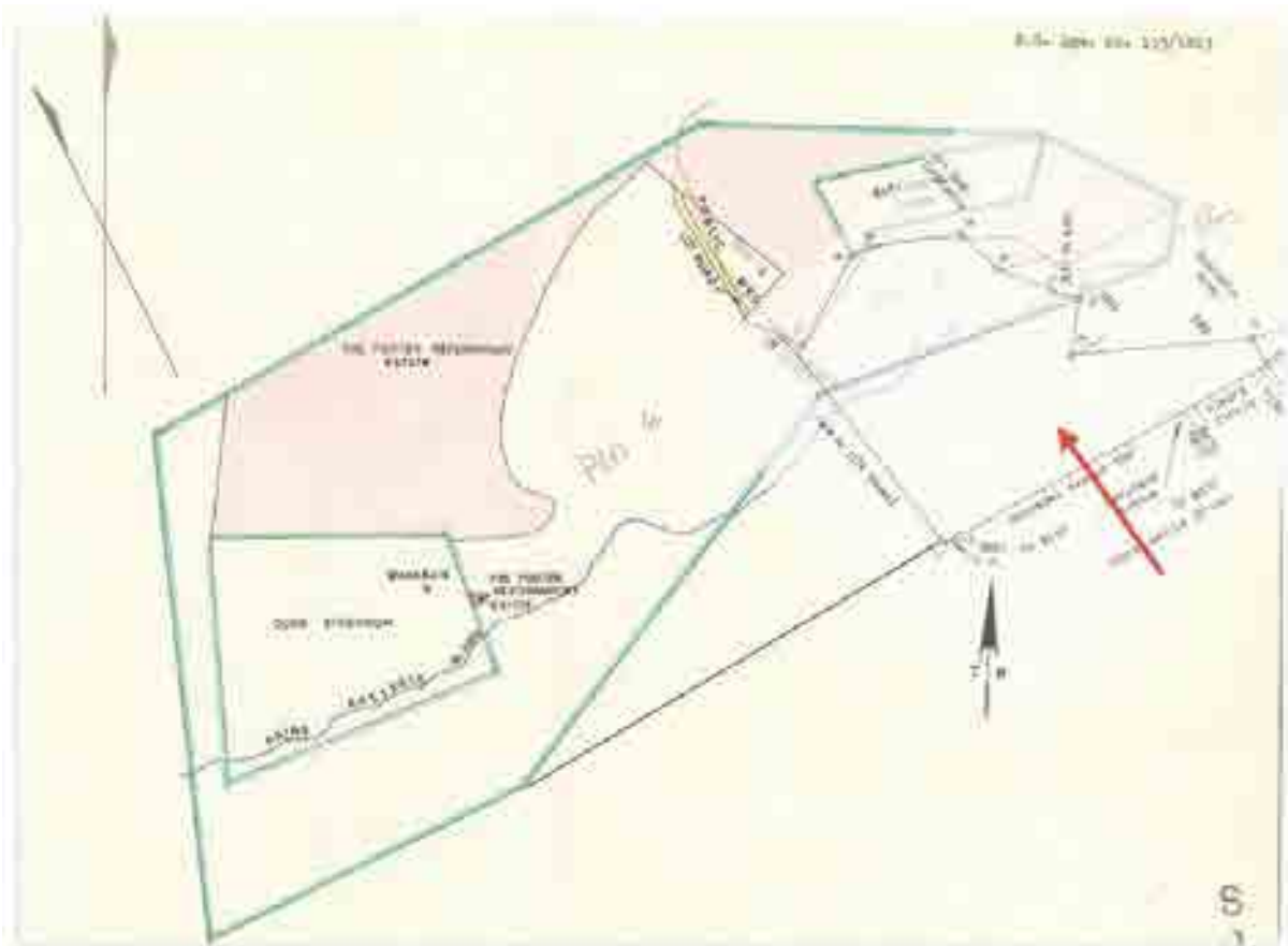
Figure 1: A survey diagram of 1996 superimposed on SGD Diagram 113/1813, showing where the Prinskasteel canal ended in the Lower Tokai Park, according to the 1813 survey. The depiction of the watercourse is accurate, given the accuracy of the original survey diagram. Subsequent annotations include subdivision for the Porter Reformatory in 1918.
